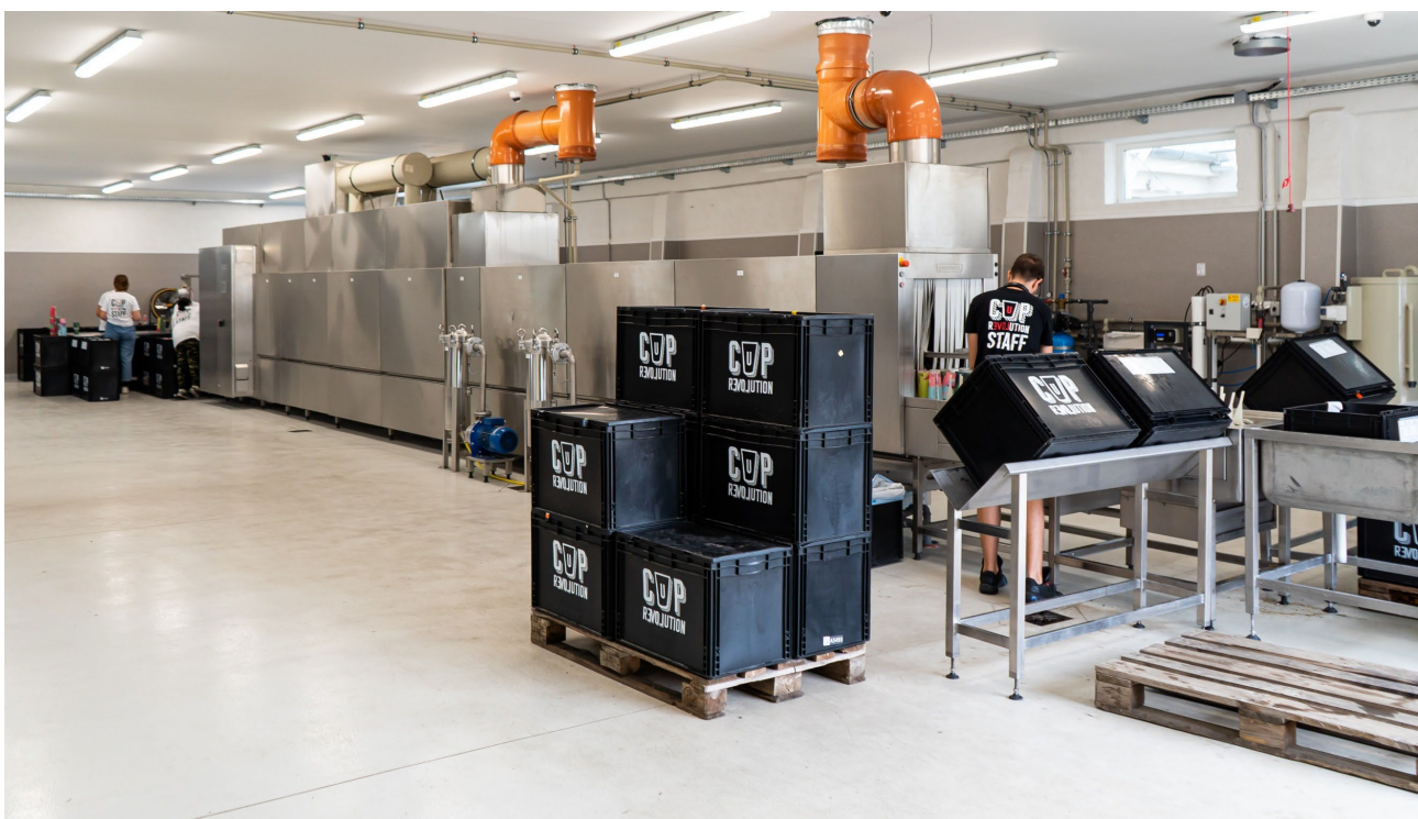
Picture 4 The industrial dishwasher used for cleaning the products at the headquarter of Revo Union
